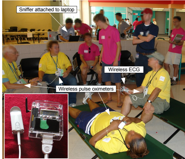
Figure 3: The indoor treatment area of the disaster drill. Faces are blurred to preserve anonymity. Inset shows the electronic triage tag, consisting of an MSP430 processor, CC2420 radio, status LEDs, display, and pulse oximeter for measuring patient vital signs.
