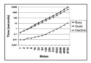
Figure 12: Scalability of TOSSIM on three applications as a function of the number of motes. *Each simulation ran for ten virtual seconds*.
