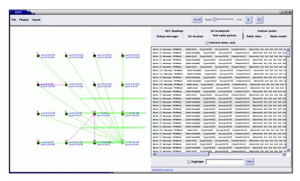
Figure 6: TinyViz connected to TOSSIM running an object tracking application. The right panel shows sent radio packets, the left panel exhibits radio connectivity for mote 15 and network traffic. The arrows represent link quality and packet transmissions.
