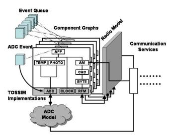
Figure 3: TOSSIM Architecture: Frames, Events, Models, Components, and Services
