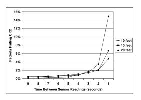
Figure 9: Packet CRC Failure Rates in Surge for Three Network Densities and Varying Sensing Frequencies. Each line shows a different network density, specified by the spacing between nodes in a 5x5 grid.
