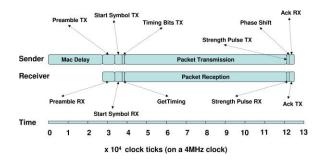
Figure 7: TinyOS Packet Sending/Reception
