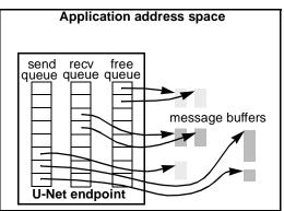
Figure 1: U-Net building blocks. *Endpoints* serve as an application's handle into the network, *buffer areas* are regions of memory that hold message data, and message queues (*send/recv/free queues*) hold descriptors for messages that are to be sent or that have been received.
